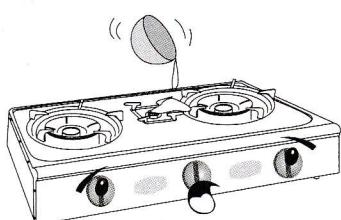
4. Protect the electric ignition system from liquid spill.
